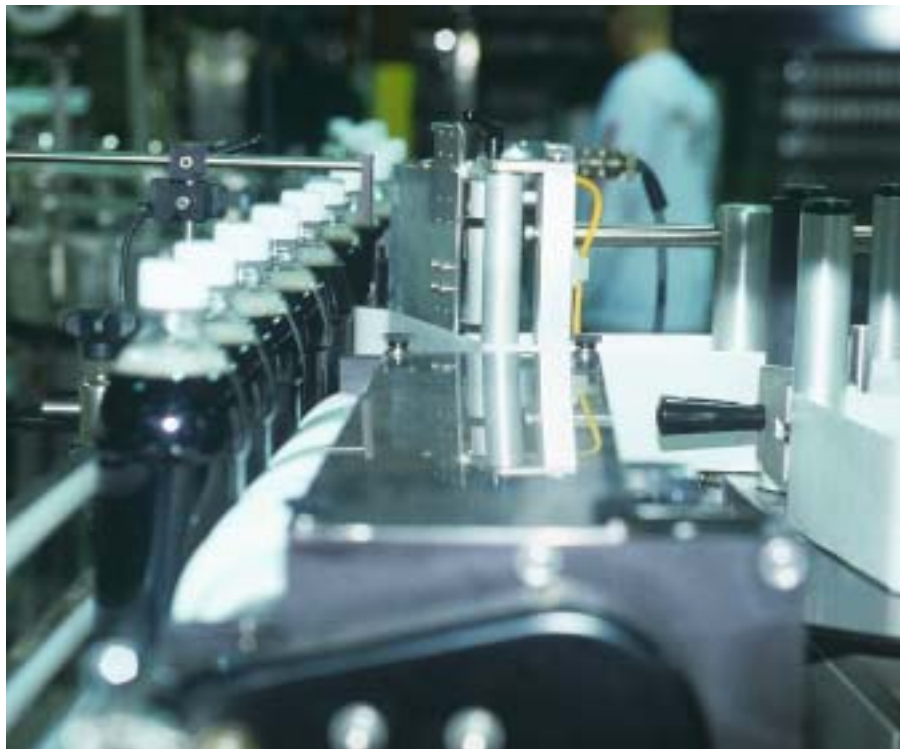
Bottles index single file from front to back through a timing screw before a label is wiped on.
