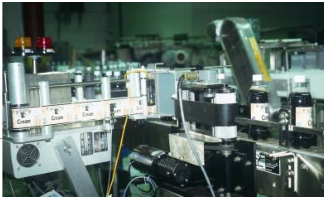
Label rollstock unwinds through a series of dancer rollers. After labeling, bottles discharge single file to a tray-packing station.
