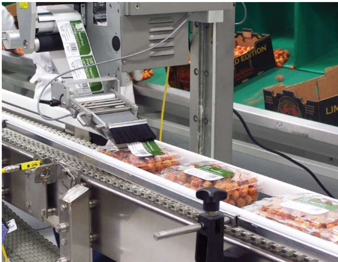
SPEEDIER APPLICATION. Pressure-sensitive labels are applied to the tops of the clamshells at approximately 50/min.
