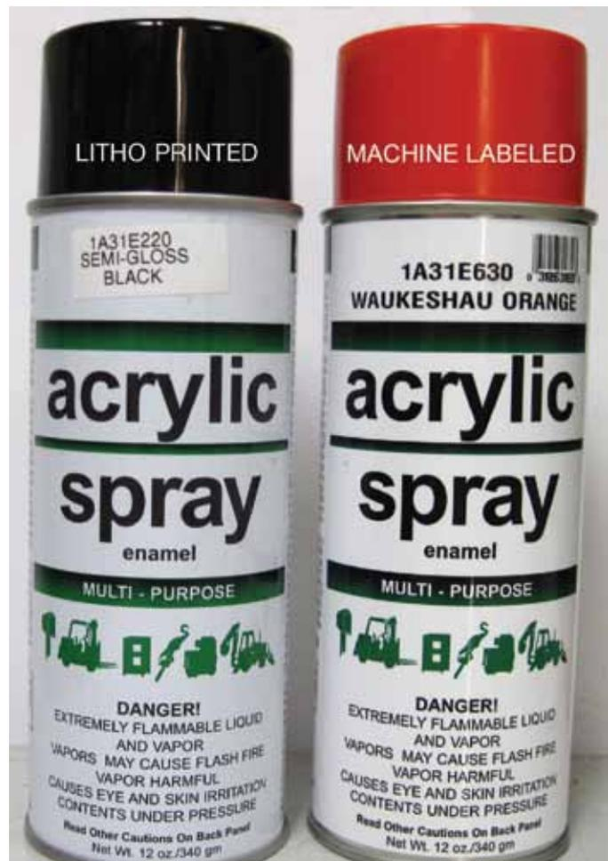
**VERSATILE PRINTING.** Variable label information is printed on demand so no additional stickers need to be manually applied to the cans.
