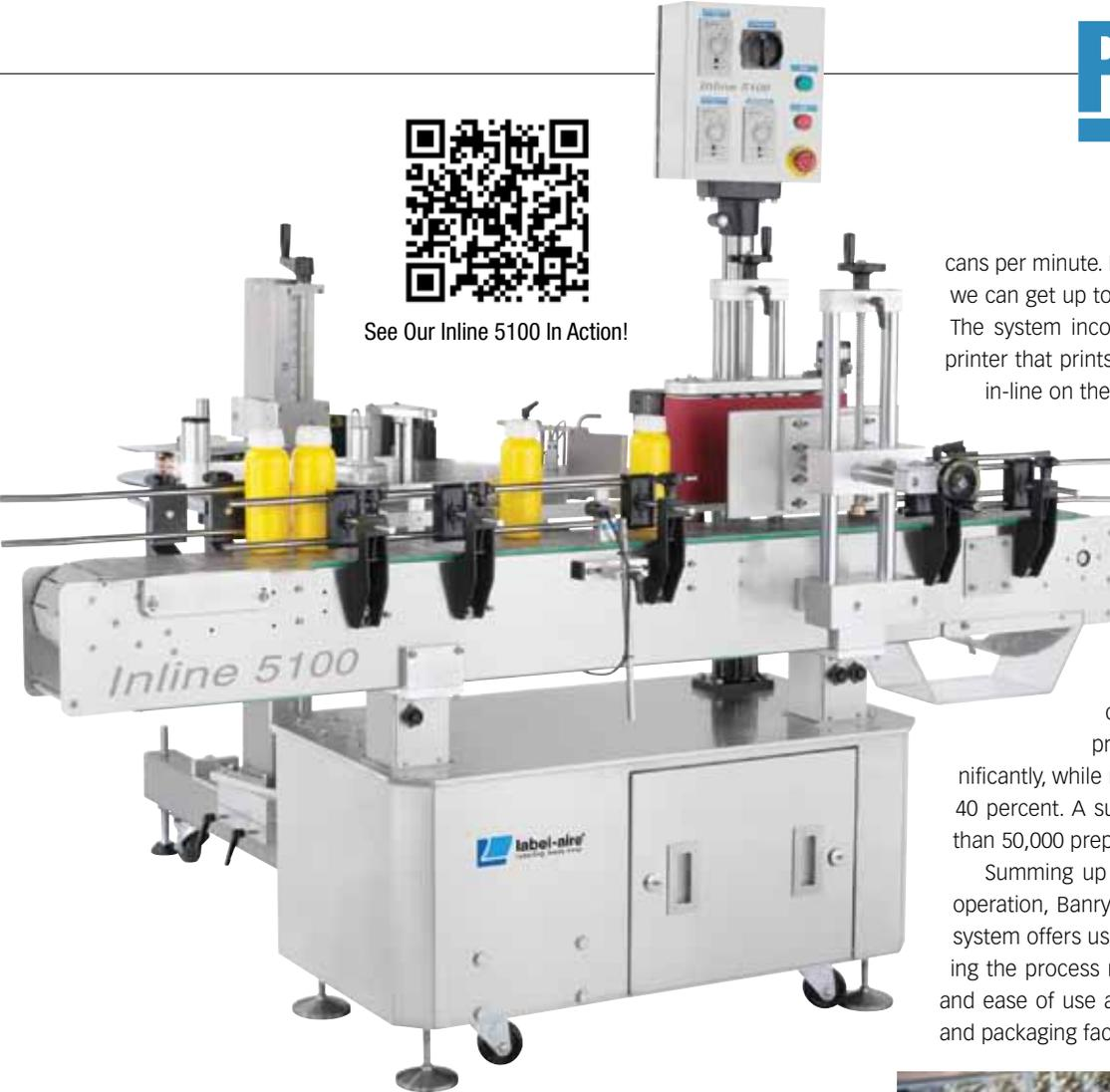
cans per minute. But with some adjustments, we're confident that we can get up to 65 cans per minute with the Label-Aire system. The system incorporates a Zebra Technologies thermal-transfer printer that prints bar codes, date codes, and other variable data in-line on the pressure-sensitive labels.
