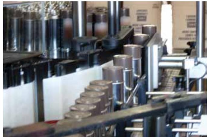
**IT'S A WRAP.** The pressure-sensitive wrap labels are automatically applied to the paint cans at current speeds of about 45 cpm.
