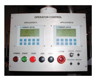
The panel controls both applicator heads and can pivot 270° for operator ease.
