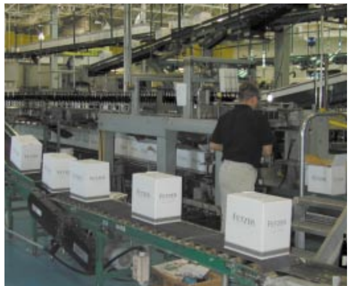
Print-and-apply systems are set up at the end of each production line.
