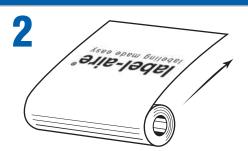
Design printed **across** roll. **Bottom** of design leading into machine.
