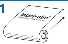
Design printed **across** roll. **Top** of design leading into machine.
