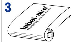
Design printed **with** the roll. **Right-hand** side of design leading into machine.
