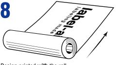
Design printed with the roll. Left-hand side of design leading into machine.
