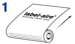
Design printed **across** roll. **Top** of design leading into machine.
