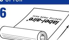
Design printed **across** roll. **Bottom** of design leading into machine.
