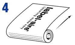
Design printed with the roll. Left-hand side of design leading into machine.
