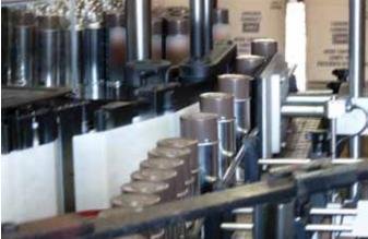
IT'S A WRAP. The pressure-sensitive wrap labels are automatically applied to the paint cans at current speeds of
